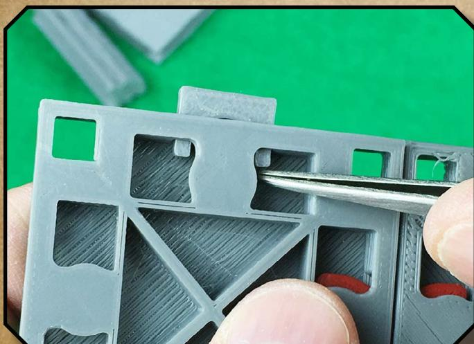
To remove a plug, insert a thin tool (like tweezers) behind it and gently push forward.
