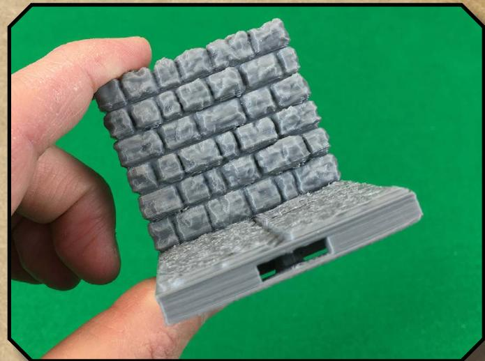
Before inserting a Dragonbite™ clip, you must first remove the printing support present in each slot on all four sides of every model. We recommend using needle-nose pliers to gently twist the support out of place (always wear eye protection when using tools.) Clips should be printed with 15-20% infill (but can be printed with 0%.)
