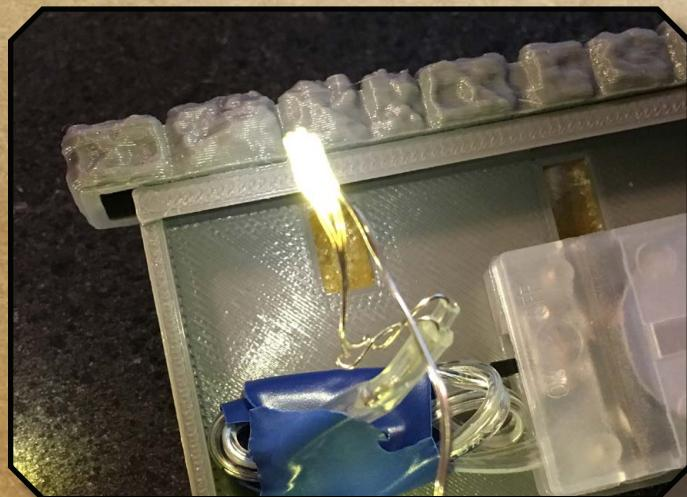
For each LED, bend the wires as much as possible to the rear of it, this will help when inserting them into the torch flames. You can insert between 1 to 3 LED bulbs per flame. Fewer bulbs mean longer battery life, but three bulbs look incredible.
