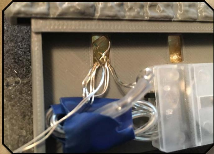
Here is the first torch flame socket with three LEDs inserted. It helps to push the LED into the socket one at a time, using tweezers to shove them inside. Once you have the LEDs inserted, apply electrical tape over the area to keep them from coming out of the socket (you can use hot glue, too.)
