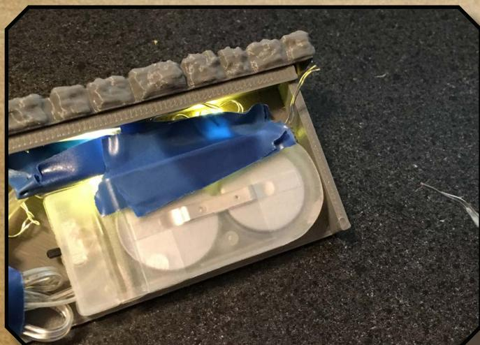
When done, you can simply cut off the remaining strand of LED bulbs. You can opt to not do this, and leave them tucked inside the wall, but this will drain your battery faster.
