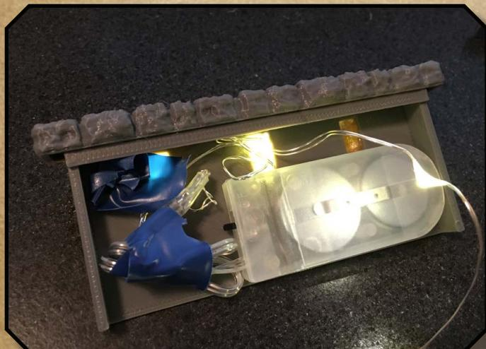
Proceed with the following two flame sockets, tapping each shut after the LEDs are inserted. It helps to have the LED's on while inserting them so you can see their position easier and be sure you are happy before taping them in place.
