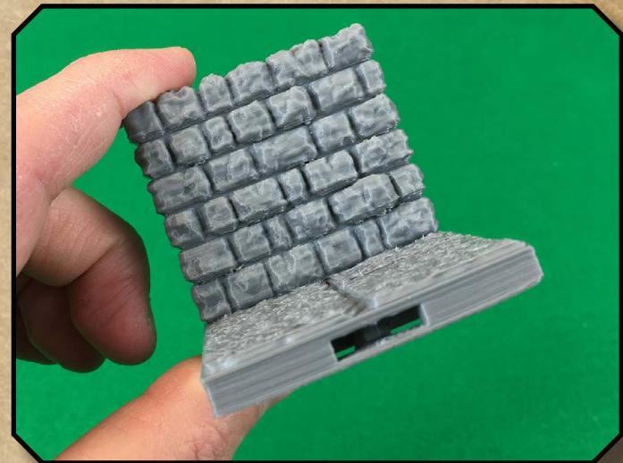
Before inserting a Dragonbite™ clip, you must first remove the printing support present in each slot on all four sides of every model. We recommend using needle-nose pliers to gently twist the support out of place (always wear eye protection when using tools.) Clips can be printed with 0% infill, but 15-20% is better.
