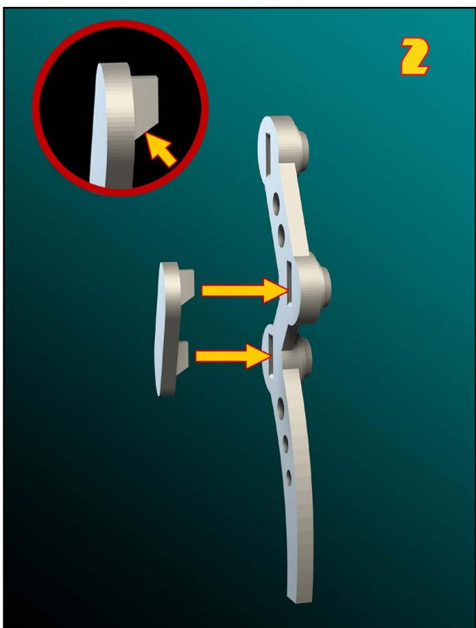
Step 2: Note that the tabs have an angled edge on the LOWER SIDE. If the angled side of the tab is on the top, you have the part upside down.
