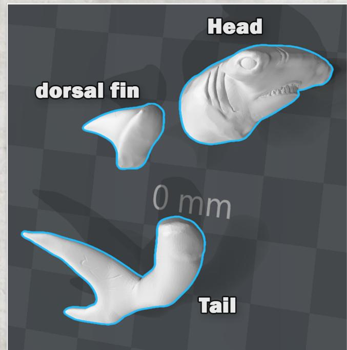
Rotate and align the model to find the best angle to print it with support. Use brim around the object.
