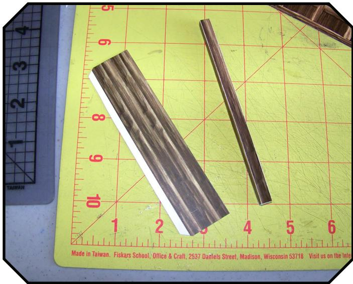
1: Cut, score and test fold the four support beam pieces as shown above. Glue together and set aside until the upper floor is finished.
