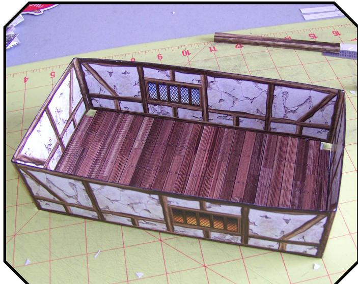
7: Once the inner walls are dry, insert and glue the floor into place. The upper floors need to have the four corner squares cut out first. For the upper floor, before gluing the piece into place, cut out a 1x2 square section wherever you want the opening for the stairs to be (make sure it's over the first floor area and not the extension.)
