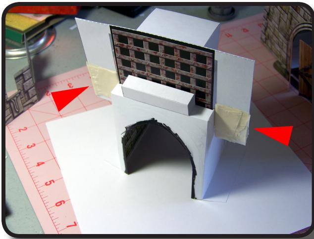
Step 5: Fold the portcullis in half and glue. When dry, wrap marking tape around the outer arms and insert into the interior assembly as shown. If the gate slides down on its own add more tape as necessary to increase resistance. The gate should stay at any position you place it at due to friction created by the tape.
