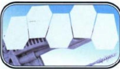
7. Now for the tricky bit! Before gluing the hull field generator plates **H2** into place, take a file and roughen up the lower hull and the edges of the upper hull slightly. This is to make gluing the plates on easier. For a final check to make sure the pieces line up well and sit in place, do a dry run, sticking them in place with blue tac. Stagger the fit as
