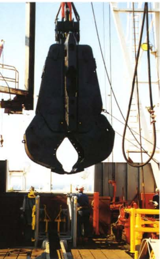
ABOVE: The giant intelligent grab, designed and built by IFREMER, was equipped with thrusters and cameras to enable it to be deployed accurately on the seabed to within a few inches. The drill pipe from which it was suspended meant that the grab could exert approximately one hundred tons of pulling power.
