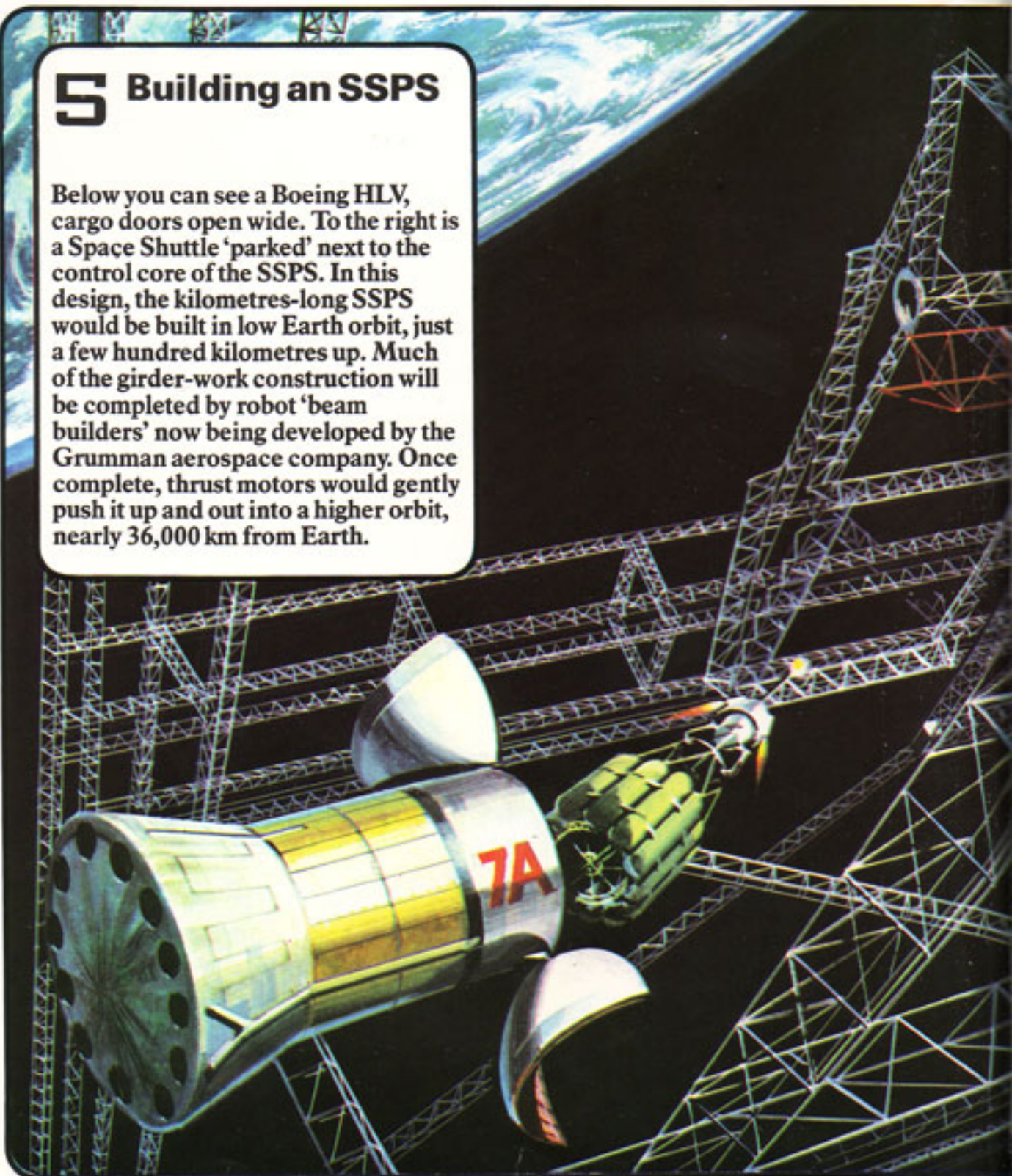
▲ This dumpy-looking spaceship is the Boeing aircraft company's idea of a Heavy Lift Vehicle of the 1990s. With a mighty roar the HLV takes off, loaded with up to 227 tonnes of cargo. Its destination, a 'building site' in orbit.
