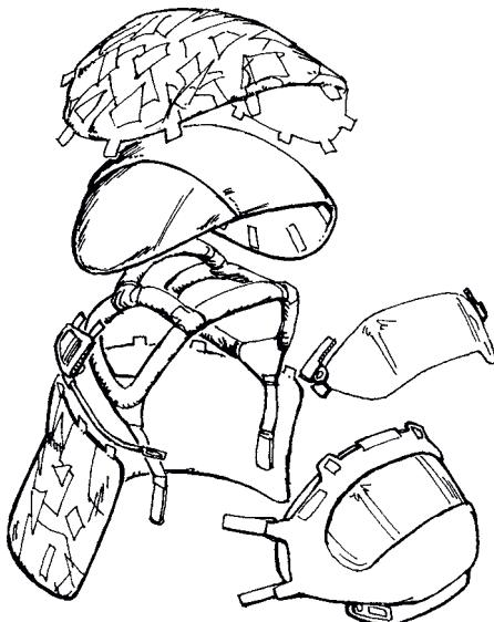
Lightweight and durable, the standard EDF battle helmet is designed to protect against impacts and shrapnel, as well as keep an infantryman in constant contact with the chain of command. The rigid monomolecular shell can deflect direct hits from smaller caliber sidearms, and internal padding diffuses the shock of impacts. The
