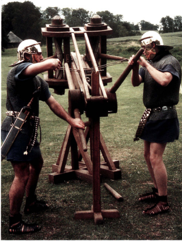
The ballista belonging to the Ermine Street Guard re-enactment group is the optimum size to launch stones weighing around 4 Roman pounds (1.3kg). Even such a lightweight catapult requires considerable space to operate efficiently. (© Ermine Street Guard)
