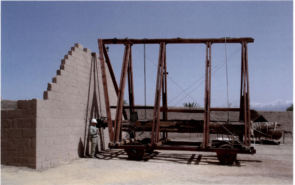
A reconstruction of the ram-tortoise described by Apollodorus of Damascus. The outer cladding of timber and wickerwork, covered with a fireproof layer of clay, has been omitted, so that the frame and undercarriage can be seen. (© P. Slisz)
