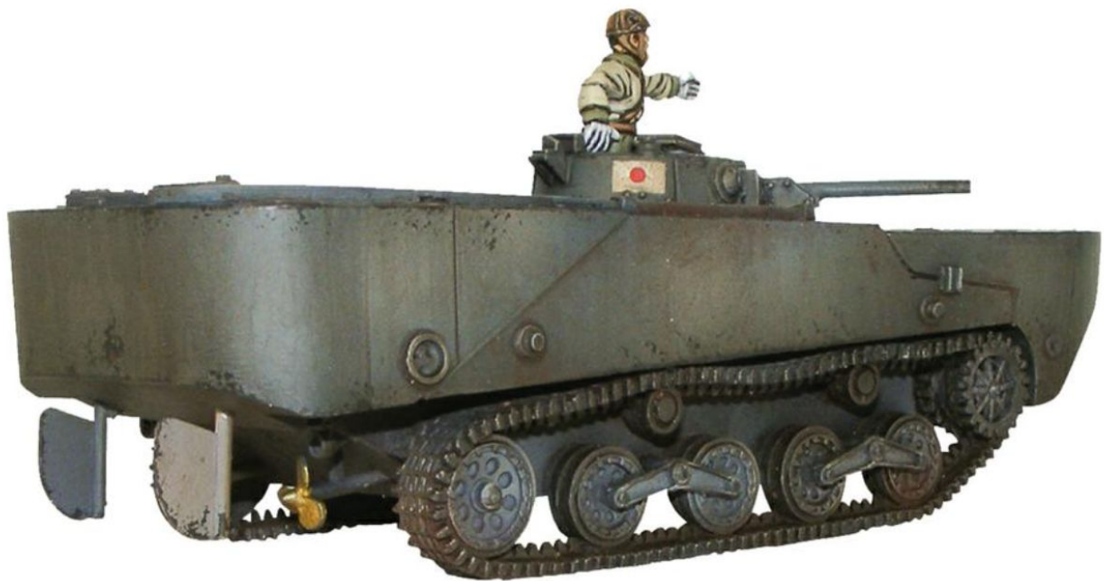
Type 2 Ka-Mi amphibious tank with floating pontoons still attached
