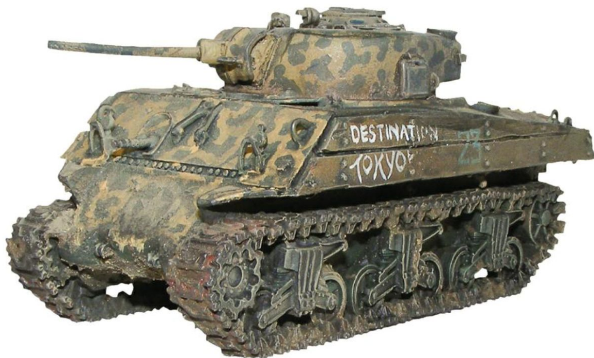
M4A3 Sherman with wooden side armour
