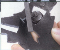
The contact points on the hull and belly plate were filed down to the bare plastic to ensure a strong bond.
